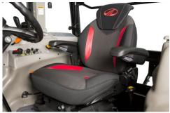
**AIR SUSPENSION SEAT** 9000 series tractors come standard with the mComfort Air Ride seat, featuring adjustable armrests and headrest, to reduce operator fatigue and increase productivity.
